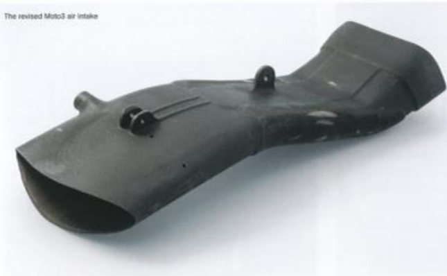
The revised Moto3 air intake
