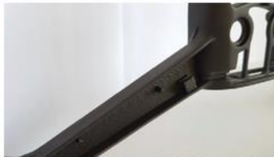
Reinforced composite materials are used in 3D printing parts for the Bebop 2 quadcopter.
