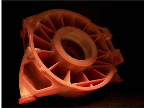
*Picture 1: Disposable pattern: laser sintering and red wax infiltration*
