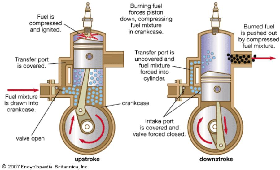
Picture 5: The performances of a two-stroke engine
