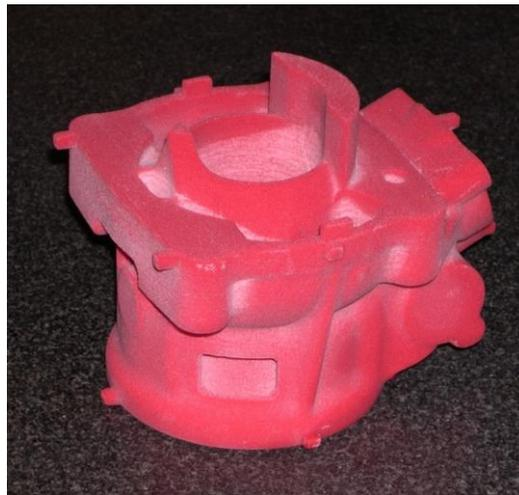
*Picture 8: A disposable pattern of the cylinder is made through RP techniques and the new Windform® PS.*
