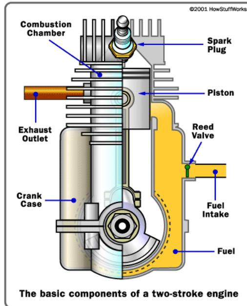
*Picture 4: The basic components of a two-stroke engine*
