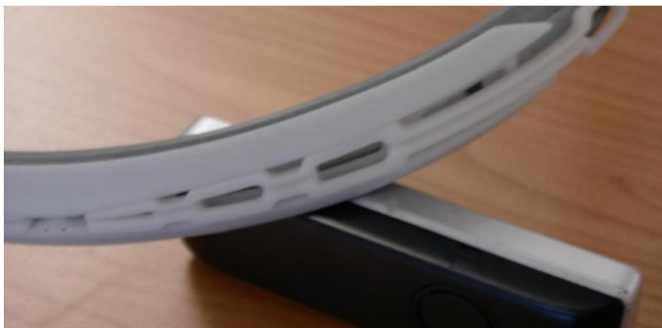
Picture 4: the bumper made in Windform FX
