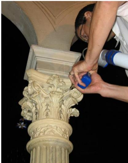
When measuring was finished, the three dimensional point cloud was transformed into a 3D mesh in .stl format.
