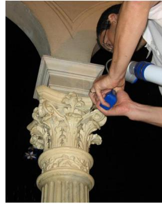
2. The file coming from the scanning system has to be optimized using filters and tools inside the reverse engineering software. Different point clouds, coming from different measuring sessions, are aligned in the same reference system while the double points, that are captured during the sessions more than one time, are deleted.
