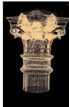
3. The following step is to generate a STL model, showing the object surfaces with a triangular faced three-dimensional mesh. This file can be sent to rapid prototyping machines to manufacture copies of the original model, it can be exported in graphic formats for video presentation (3D rendering) or it even can be saved to generate the database of the parts digitized.
