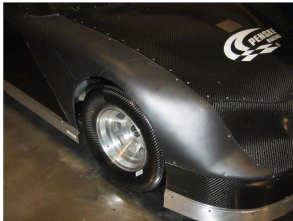
During wind tunnel run, as usually a map of various ride height with each of these component, the carbon fibre one then the WINDFORM<sup>®</sup> XT one, and standard aero parameters have been measured on the model, drag, lift ( = downforce ) and balance allowing full post session analyse for others aero parameter like efficiency.
