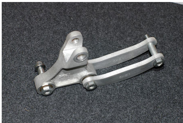
Picture 3a/b – Link elements of the Yamaha TZ250 2005. Notice the cast triangle and the connecting rod divided into two drop-forged pieces. The elements are in aluminium.
