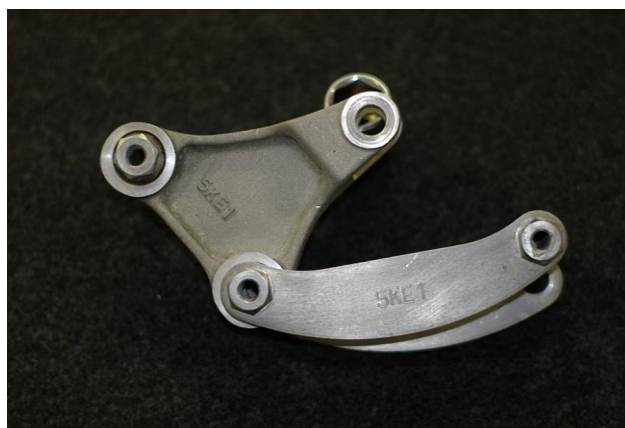
Picture 3a/b – Link elements of the Yamaha TZ250 2005. Notice the cast triangle and the connecting rod divided into two drop-forged pieces. The elements are in aluminium.
