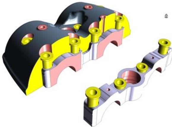
Then everything is assembled on a specific "jig" (mask) with the use of high performing adhesives developed for strong aerospace applications, with maximum confidentiality on their composition and properties.
