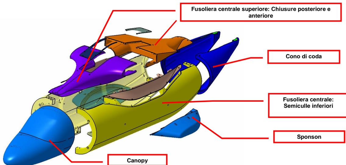
**Exploded view of the external fairings made in WINDFORM GF**
