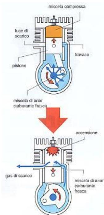
**1. Compression/intake:** The air/fuel/oil mixture has entered the cylinder, and the piston begins to move up. This compresses the charge in the cylinder and draws a vacuum in the crankcase, pulling in more air, fuel, and oil from the carburetor. The compressed charge is ignited by the spark plug, and the cycle begins again.
