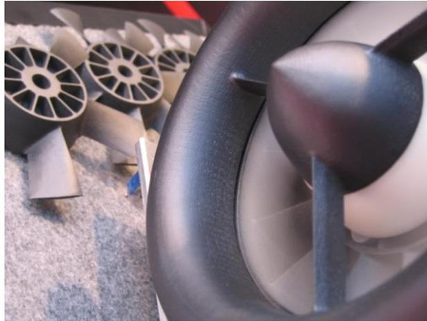
Coupling the fan to the mini double flow turbojet, you end up with the above mentioned double flow turbofan, with much higher thrust values (you can reach 6/7 Kg) but, thanks to the compressor performance, it would guarantee extremely low specific consumption values (that's why turbofans are used on commercial aircrafts).
